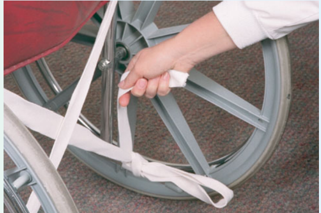
▲ Pull end of tie and loosen first crossover tie in an emergency.
