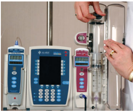
4 Anchor syringe/plunger in three steps; be sure plunger is anchored according to manufacturer's directions.
