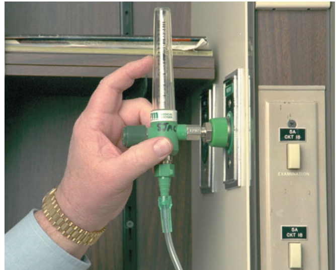
▲ Oxygen flow meter indicates liters per minute delivered to administration setup.
