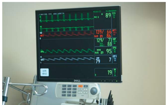
▲ Monitor displays digital readouts and pressure waveforms of the ECG, arterial BP, SPO 2 and calculated CPP ( \text{MAP} - \text{ICP} = \text{CPP} ).
